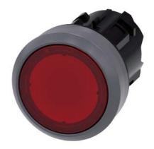
Illuminated pushbutton, 22 mm, round, plastic with metal front ring, red, pushbutton, flat, latching, Push-to-release mechanism, with laser labeling, symbol number according to, ISO 7000 or IEC 60417
