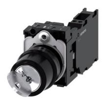
RONIS key-operated switch, 22 mm, round, plastic, lock number SB30, with 2 keys, 2 switch positions O-I, latching, 10:30h/13:30h, key removal O+I, with holder, 1 NO+1 NC, spring-type terminal, possible special locks: SB31, 421, 455, with laser labeling, upper case
