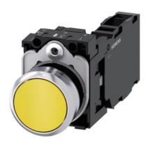
Pushbutton, 22 mm, round, metal, shiny, yellow, pushbutton, flat, momentary contact type, 1 NO+1 NC, screw terminal, with laser labeling, upper case and lower case, always upper case at beginning of line
