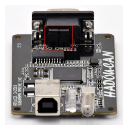
Internal termination resistors can be selected by inserting 2x 0.1in jumpers onto pins 1&2 and 3&4 of J2, located adjacent to the DE9 connector. This will connect a 120 ohm split termination right after the D Sub connector. The device ships from the factory with the termination enabled.
