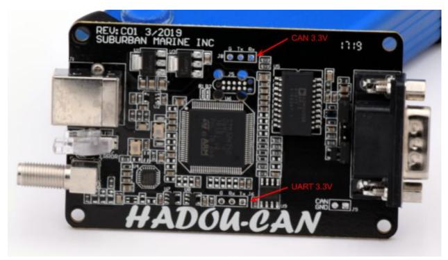
A 3.3V logic level UART is present on J6 that will output boot and diagnostic messages. A 3.3V logic level CAN header, J8, is also present, which can be used as a logic analyzer or oscilloscope connection point. The CAN header is useful for diagnosing bit rate issues and verifying loop delay time.
