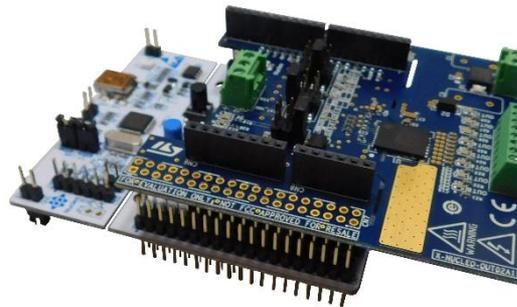
X-NUCLEO-OUT02A1 plugged on to a compatible STM32 Nucleo board
