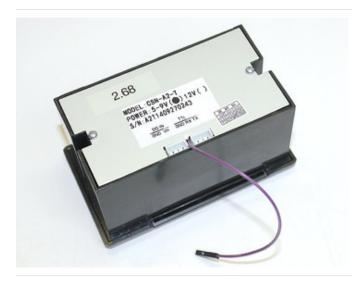
Screw the controller board back in place (check that neither of the cables has come unseated), routing the DTR wire around between the two sockets, then screw the back on.
