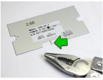
On the back plate, there's a small metal "finger" between the serial and power sockets. Using pliers, this can be bent back to provide an exit route for the DTR wire.
