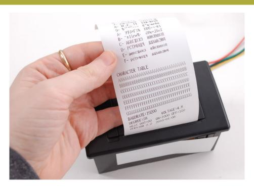
If you don't get a printout, check that the paper is inserted correctly and not binding, that the power is correctly wired, power supply is plugged in, etc. Then try again, holding down the button when connecting power.
