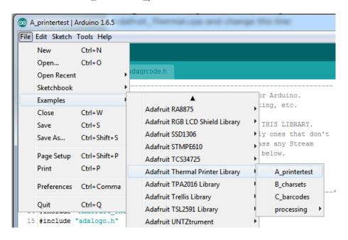
If your printer test page shows 'BAUDRATE: 9600', you'll need to make a small change to the library source code. Using a text editor (Notepad, etc.) open the file Adafruit\_Thermal.cpp and change this line:
