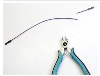
Cut an end off a female jumper wire and strip & tin the end.
