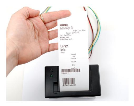
If this does not work, first check that the printer and Arduino are both powered, and that the data in, out and ground wires are properly connected to the Arduino.
