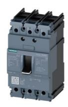
circuit breaker 3VA5 UL frame 125 breaking capacity class S 25kA @ 480 V 3-pole, line protection TM210, FTFM, In=90A overload protection Ir=90A fixed short-circuit protection Ii=10 x In nut keeper kit on both sides
