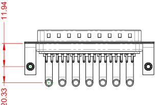
**OPERATING TEMPERATURE:** -55°C ~ 125°C 40A (CURRENT) POWER/CO-AX CONTACT RATING: (IF PRESENT) SIGNAL CONTACT CURRENT RATING: 5A PER CONTACT SIGNAL CONTACT RESISTANCE:  $10m\Omega$  MAX. **INSULATOR RESISTANCE:** 5000MΩ min. DIELECTRIC
