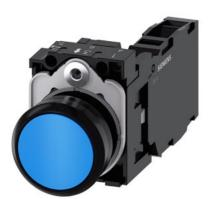
Pushbutton, 22 mm, round, plastic, blue, pushbutton, flat, momentary contact type, with holder 1 NO+1 NC, screw terminal, Z=20-unit packaging
