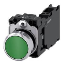
Pushbutton, 22 mm, round, metal, shiny, green, pushbutton, flat, momentary contact type, 1 NO+1 NC, spring-type terminal, with laser labeling, symbol number according to, ISO 7000 or IEC 60417
