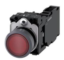
Illuminated pushbutton, 22 mm, round, plastic with metal front ring, red, pushbutton, flat, momentary contact type, with holder, 1 NO+1 NC, LED module with integrated LED 230 V AC, screw terminal, with laser labeling, inscription or symbol Customer-specific selection with SIRIUS ACT configurator (CIN)
