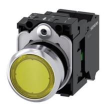
Illuminated pushbutton, 22 mm, round, metal, shiny, yellow, pushbutton, flat, momentary contact type, with holder, 1NO, LED module with integrated LED 110 V AC, spring-type terminal, with laser labeling, inscription or symbol Customer-specific selection with SIRIUS ACT configurator (CIN)
