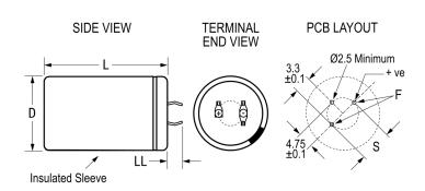
General Information Series ALC80 Dielectric Aluminum Electrolytic Description Snap-In, Aluminum Electrolytic RoHS Lead 3 Pin Short AEC-Q200 No Halogen Free Yes Component Weight 35 g Notes Dimensions D And L Include Sleeving. Shelf Life 156 Weeks
