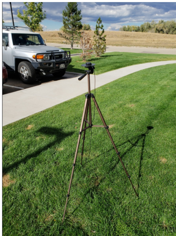
GNSS antenna sitting on a metal ground plate elevated with clear view of the sky
