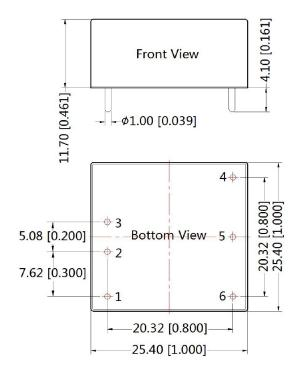
Note: Unit: mm[inch] Pin diameter tolerances: ±0.10[±0.004] General tolerances: ±0.50[±0.020] Note:Grid 2.54\*2.54mm
