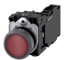
Illuminated pushbutton, 22 mm, round, plastic with metal front ring, red, pushbutton, flat, momentary contact type, with holder, 1 NO+1 NC, LED module with integrated LED 230 V AC, screw terminal, with laser labeling, upper case
