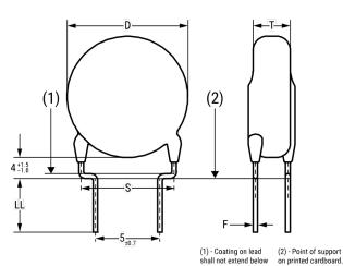
(1) - Coating on lead shall not extend below this line.
