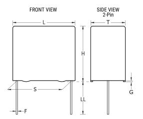
**General Information** Series F611 Dielectric Metallized Polyester Style Radial MKT (Wound), DC Multipurpose Applications Features RoHS Yes Lead Wire Leads AEC-Q200 No Component 5.909 g Weight The Rated Voltage Decreases 1.25%/C Between +85C And +105C (For +125C, Please Consult KEMET). ClimCat: 55/105/56. Miscellaneous
