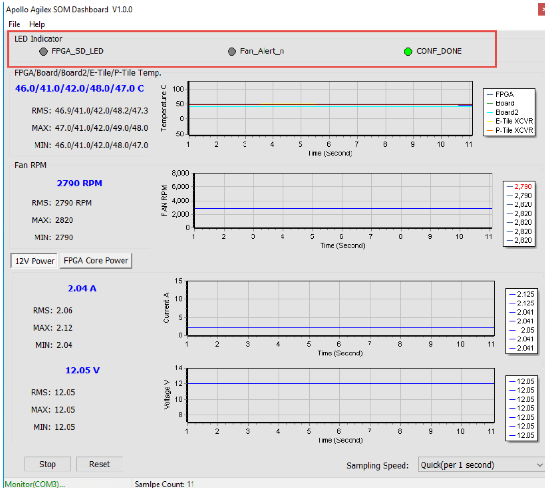
Figure 3-5 FPGA Status section
