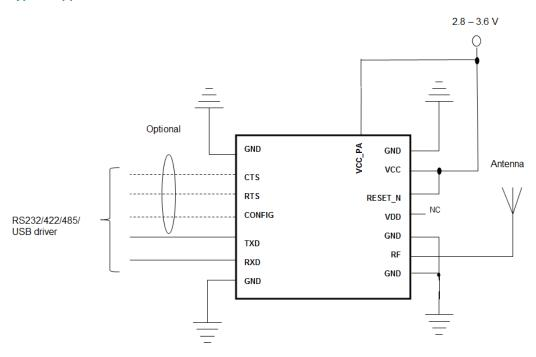
Note that the VCC\_PA pin supply the internal power amplifier only while the rest of the internal block runs on VCC. They can be connected together or separated using individual supply.
