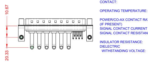
30A (CURRENT) POWER/CO-AX CONTACT RATING: (IF PRESENT) SIGNAL CONTACT CURRENT RATING: 5A PER CONTACT SIGNAL CONTACT RESISTANCE:  $10m\Omega$  MAX. **INSULATOR RESISTANCE:** 5000MΩ min. DIELECTRIC
