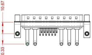
20A (CURRENT) POWER/CO-AX CONTACT RATING: (IF PRESENT) SIGNAL CONTACT CURRENT RATING: 5A PER CONTACT SIGNAL CONTACT RESISTANCE:  $10m\Omega$  MAX. **INSULATOR RESISTANCE:** 5000MΩ min. DIELECTRIC
