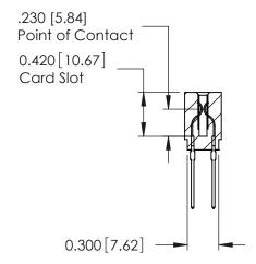
725 Series Ultra-Mate Card Edge Connector - Press Fit
