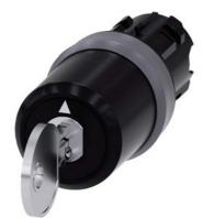
key-operated switch Siemens, 22 mm, round, plastic with metal front ring, lock number SSG10, with 2 keys, 3 switch positions I-O-II, latching, actuating angle 2x45°, 10:30h/12h/13:30h, key removal O, with laser labeling, upper case
