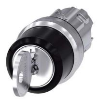
RONIS key-operated switch, 22 mm, round, metal, shiny, lock number SB30, with 2 keys, 3 switch positions I>O<II, momentary contact type, actuating angle 2x45°, 10:30h/12h/13:30h, key removal O, possible special locks: SB31, 421, 455, Z=50-unit packaging
