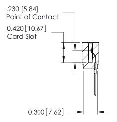
725 Series Ultra-Mate Card Edge Connector - Press Fit DRAWN: Part Number: 725-021-540-101 **EDAC INC** THESE DRAWINGS AND SPECIFICATIONS
