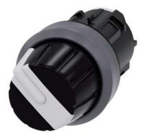
Selector switch, 22 mm, round, plastic with metal front ring, white, Rotary knob, 4 switch positions I-II-III-IV, latching, Actuating angle  $4x90^\circ, 3h/6h/9h/12h,$  with laser labeling, upper case and lower case, always upper case at the beginning of the word
