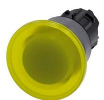
Illuminated mushroom pushbutton, 22 mm, round, plastic with metal front ring, yellow, 40 mm, momentary contact type, with laser labeling, symbol number according to, ISO 7000 or IEC 60417
