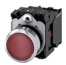
Illuminated pushbutton, 22 mm, round, metal, shiny, red, pushbutton, flat, momentary contact type, with holder, 1NC, LED module with integrated LED 24 V AC/DC, screw terminal, with laser labeling, symbol number according to, ISO 7000 or IEC 60417
