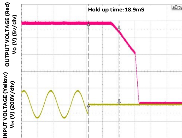
Figure 6. Typical Hold-up Waveforms ( V_{IN} = 115\text{Vac} , 100% Load)
