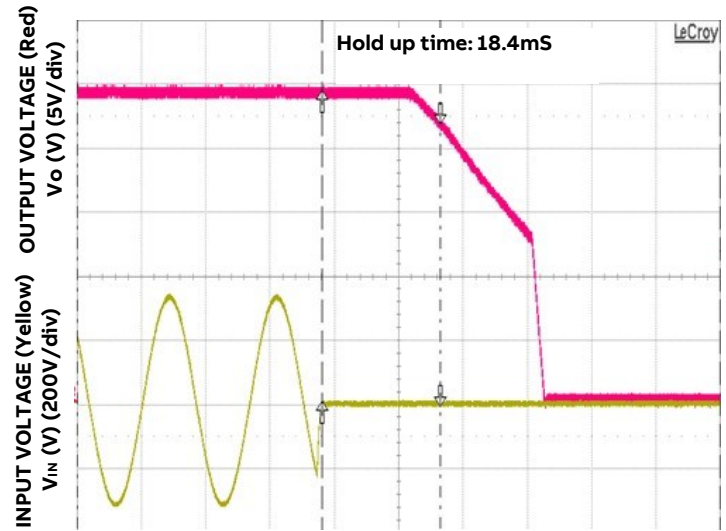
Figure 7. Typical Hold-up Waveforms ( V_{IN} = 230\text{V} , 100% Load)
