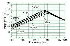
AC Line Filters - Common Mode SS Coils, 20H Series
