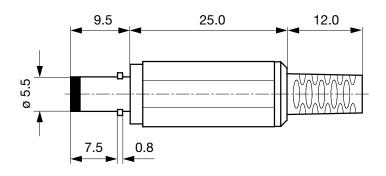
Cable diameter max. 4.0 mm
