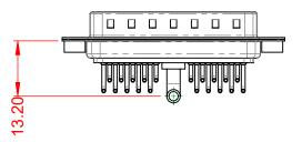
30A (CURRENT) POWER/CO-AX CONTACT RATING: (IF PRESENT) SIGNAL CONTACT CURRENT RATING: 5A PER CONTACT SIGNAL CONTACT RESISTANCE:  $10m\Omega$  MAX. INSULATOR RESISTANCE: 5000MΩ min.
