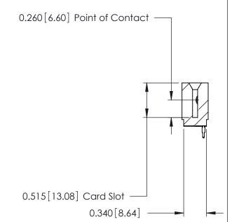
ACAD REFERENCE NO. 746-ENG MASTER 746 Series Ultra-Mate Card Edge Connector - Press Fit DRAWN: DATE: AUG 20/09 J.LEE Part Number: 746-023-520-101 CHECKED: DATE: **EDAC INC** SCALE: SHEET 1 OF 1 THESE DRAWINGS AND SPECIFICATIONS ARE THE PROPERTY OF EDAC INC., AND TORONTO, ONTARIO SHALL NOT BE REPRODUCED, OR COPIED DRAWING NUMBER **ISSUE** CANADA OR USED AS THE BASIS FOR THE 746-ENG MASTER MANUFACTURE OR SALE OF APPARATUS YOUR CONNECTION TO QUALITY & SERVICE WITHOUT WRITTEN PERMISSION.
