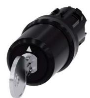
Key-operated switch BKS, 22 mm, round, plastic, lock number S1, with 2 keys, 3 switch positions I-O-II, latching, actuating angle 2x45°, 10:30h/12h/13:30h, Key removal I+II, with laser labeling, lower case
