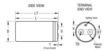
General Information Series ALS30 Dielectric Aluminum Electrolytic Description Screw Terminal, Aluminum Electrolytic RoHS AEC-Q200 No Component 690 g Weight Dimensions D And L Include Sleeving. MS (MxH) = Notes M12x16. Mounting Clamp (Sold Separately): V9ÓN Shelf Life 156 Weeks
