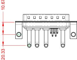
30A (CURRENT) POWER/CO-AX CONTACT RATING: (IF PRESENT) SIGNAL CONTACT CURRENT RATING: 5A PER CONTACT SIGNAL CONTACT RESISTANCE:  $10m\Omega$  MAX. **INSULATOR RESISTANCE:**
