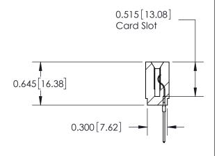
ACAD REFERENCE NOTION STEP 737 Series Ultra-Mate Card Edge Connector - Press Fit DRAWN: Part Number: 737-015-540-101 CHECKED: **EDAC INC** THESE DRAWINGS AND SPECIFICATIONS ARE THE PROPERTY OF EDAC INC.,AND TORONTO, ONTARIO SHALL NOT BE REPRODUCED, OR COPIED CANADA OR USED AS THE BASIS FOR THE YOUR CONNECTION TO QUALITY & SERVICE
