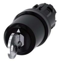
Key-operated switch IKON, 22 mm, round, plastic, lock number 360012K1, with 2 keys, 3 switch positions I>O<II, momentary contact type, actuating angle 2x45°, 10:30h/12h/13:30h, key removal O, with laser labeling, upper case and lower case, always upper case at beginning of line
