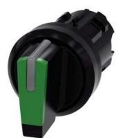
Selector switch, illuminable, 22 mm, round, plastic, green, selector switch, short, 3 switch positions I-O-II, latching, actuating angle 2x45°, 10:30h/12h/13:30h, with laser labeling, inscription or symbol Customer-specific selection with SIRIUS ACT configurator (CIN)
