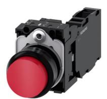
Pushbutton, 22 mm, round, plastic, red, pushbutton, raised, momentary contact type, with holder 1 NO+1 NC, screw terminal, with laser labeling, upper case
