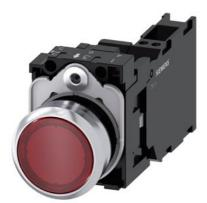
Illuminated pushbutton, 22 mm, round, metal, shiny, red, pushbutton, flat, momentary contact type, with holder, 1 NO+1 NC, LED module with integrated LED 24 V AC/DC, spring-type terminal, Z=20-unit packaging
