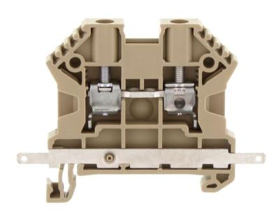
Feed-through terminal, Screw connection, Mounting type: Mounting rail TS 35/7.5, Rated cross-section: 4 mm², Width: 6 mm, Colour: Beige
