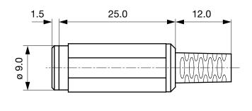
Cable diameter max. 4.0 mm
