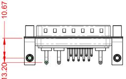
POWER/CO-AX CONTACT RATING:10A (CURRENT)(IF PRESENT)SIGNAL CONTACT CURRENT RATING:5A PER CONTACTSIGNAL CONTACT RESISTANCE:10mΩ MAX.
