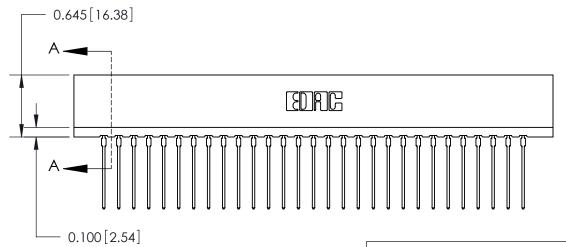
737 Series Ultra-Mate Card Edge Connector - Press Fit ACAD REFERENCE NO.
