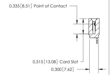
ACAD REFERENCE NO. 745 Series Ultra-Mate Card Edge Connector - Press Fit DRAWN: J.LEE Part Number: 745-044-525-101 CHECKED: **EDAC INC** SCALE: THESE DRAWINGS AND SPECIFICATIONS ARE THE PROPERTY OF EDAC INC.,AND TORONTO, ONTARIO SHALL NOT BE REPRODUCED, OR COPIED DRAWING NUMBER CANADA OR USED AS THE BASIS FOR THE 745-ENG MASTER MANUFACTURE OR SALE OF APPARATUS YOUR CONNECTION TO QUALITY & SERVICE WITHOUT WRITTEN PERMISSION.
