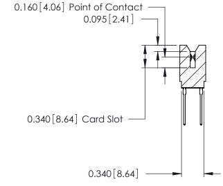
ACAD REFERENCE NO. 746 Series Ultra-Mate Card Edge Connector - Press Fit DRAWN: J.LEE Part Number: 746-046-545-606 CHECKED: **EDAC INC** SCALE: THESE DRAWINGS AND SPECIFICATIONS ARE THE PROPERTY OF EDAC INC.,AND TORONTO, ONTARIO SHALL NOT BE REPRODUCED, OR COPIED DRAWING NUMBER CANADA OR USED AS THE BASIS FOR THE 746-ENG MASTER MANUFACTURE OR SALE OF APPARATUS YOUR CONNECTION TO QUALITY & SERVICE WITHOUT WRITTEN PERMISSION.
