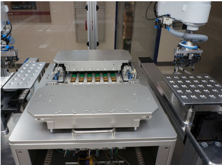
Figure 29: Automatic test equipment for module test
