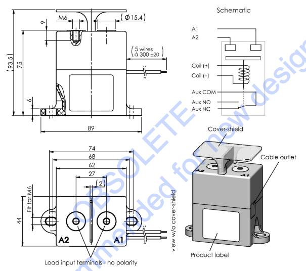
In case of no tolerance shown in dimensional drawing, general tolerances apply: dimension  $\leq 10 \, \text{mm}$ :  $\pm 0.3 \, \text{mm}$ ; dimension 10 to 50 mm:  $\pm 0.6 \, \text{mm}$ ; dimension  $> 50 \, \text{mm}$ :  $\pm 1 \, \text{mm}$
